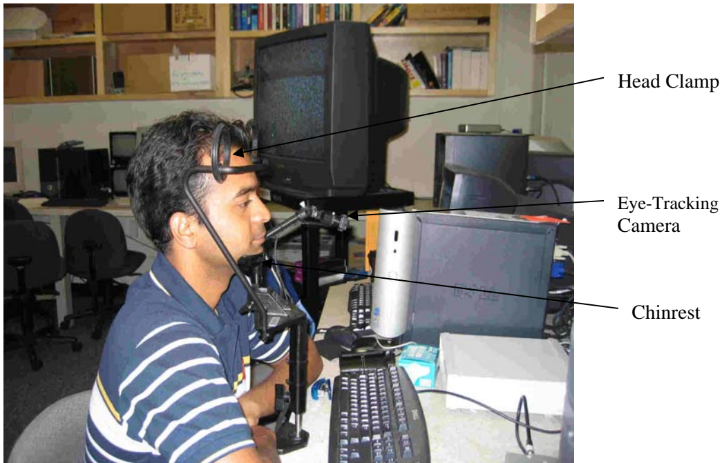
Figure 3.1 ASL Eye-Tracking Device recording user's eye-movement
