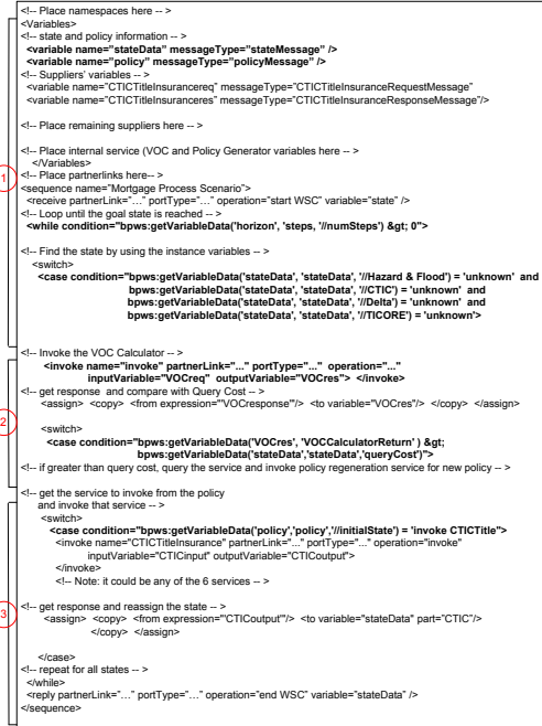
Figure 8: SOA for implementing our adaptive WSC. (a) demonstrates the interaction of the composition with internal services. In (b), we show a portion of the WS-BPEL for the mortgage acquisition process. Labels (1) (2) and (3) in (a) correspond to its associated markup in (b).
